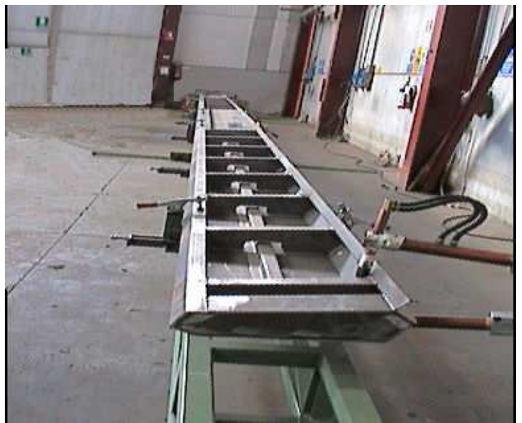
Spot welded longeron L = 17.000 mm
