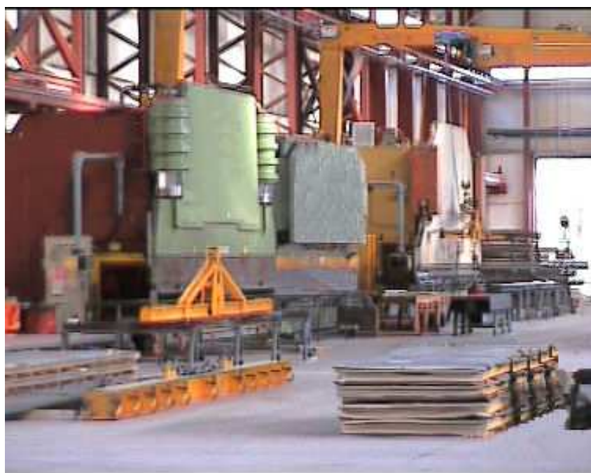
Bending and pressing line (up to 25000mm – 2500 ton)
