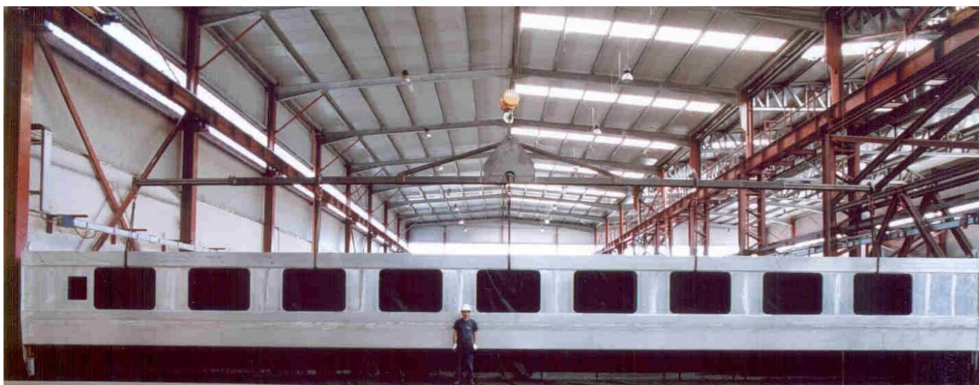
Completely automatic assembled Aluminium alloy sidewall for coaches L = 22.000 mm
