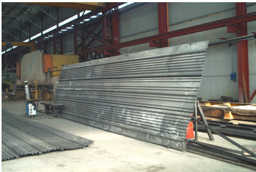
Longitudinal welded wagon's floor L = 20.000
