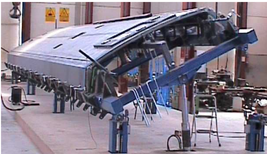
Completely assembled Wagon roof L=17.000 mm
